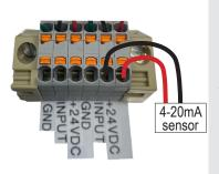
Wiring for a 3-wire sensor, powered by Yocto-4-20mA-Rx (max 80mA)
