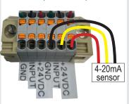
Wiring for a 4-wire sensor, with an independent power supply.
