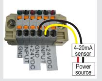
Wiring for 3-wire sensor, with independent power supply with common ground.
