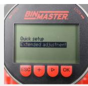
Scroll to Additional adjustments with the [>] key. Press [OK]
