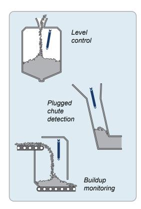
advanced algorithms to convert the timing of the pulses to a very accurate distance measurement. The sensor firmware automatically takes into account when the sensor is mounted at an angle, and adjusts the absolute distance accordingly.
