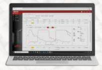
A chart showing sensor level readings converted to tons overlays the ADFI slope indicating consumption and filling, generated for a specific date range. Charts can be created based on other reading types including delivery capacity, distance, percent full, ring space, and sensor battery life. Drilling down further, the most recent sensor reading is timestamped, with reporting on all bin parameters.
