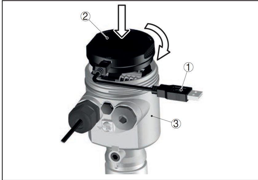
Fig. 28: Connection of the PC directly to the sensor via the interface adapter
