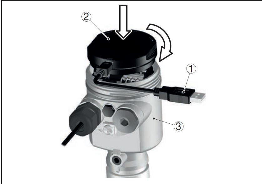
Fig. 18: Connection of the PC directly to the sensor via the interface adapter
