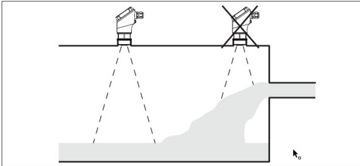
*Fig. 7: Mounting the radar sensor with inflowing material*
