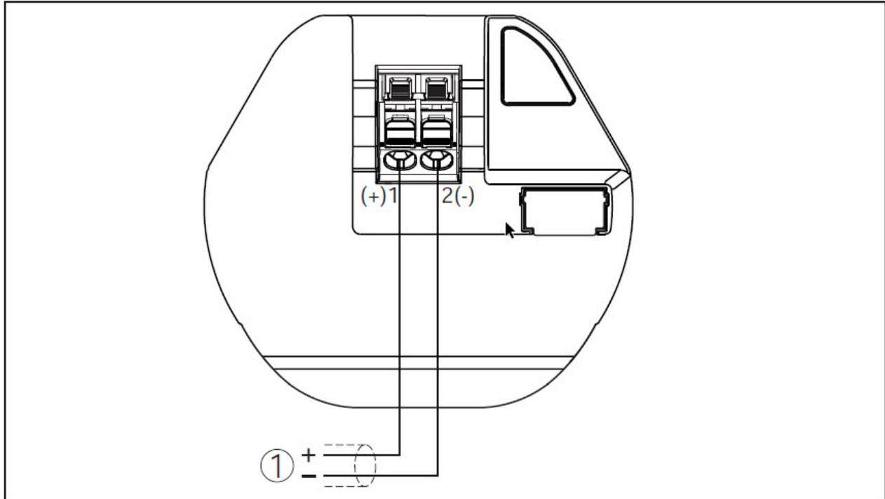
Fig. 10: Connection compartment CNCR-210/220
