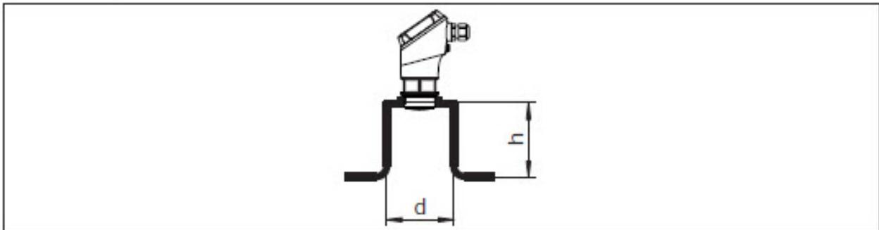
Fig. 8: Mounting the radar sensor with stand pipes
