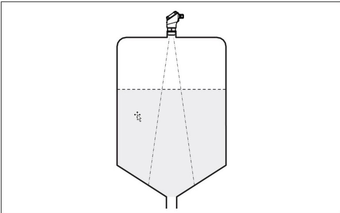
*Fig. 5: Mounting the radar sensor with conical bottom*
