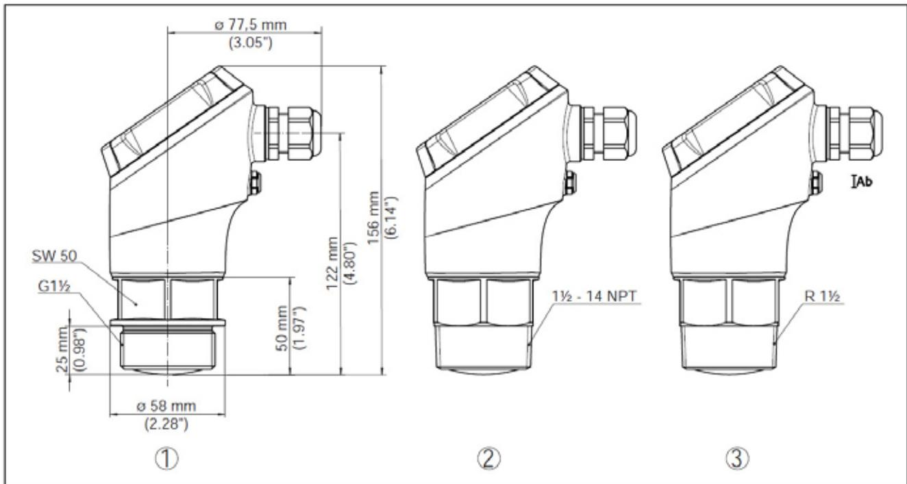
Fig. 14: Dimensions CNCR-210/220
