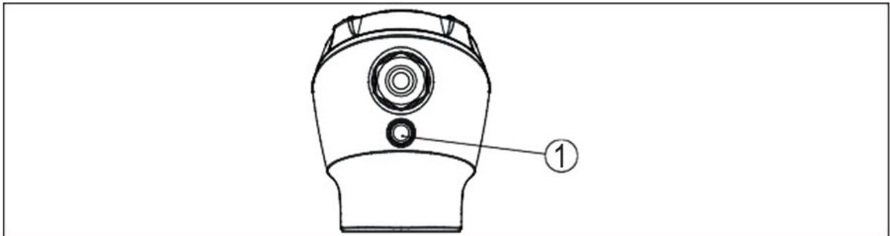
*Fig. 3: Polarization position
