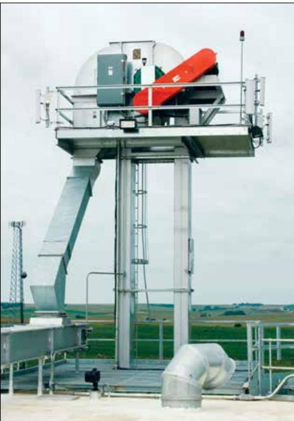
Head section of the new 20,000-bph Schlegel receiving leg from which grain can go to the new concrete storage silo.
