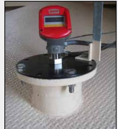
Scanner mounted on existing flange, using an adapter plate.
