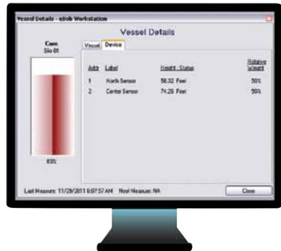
*The higher measurement at the center indicates a cone up condition.*
