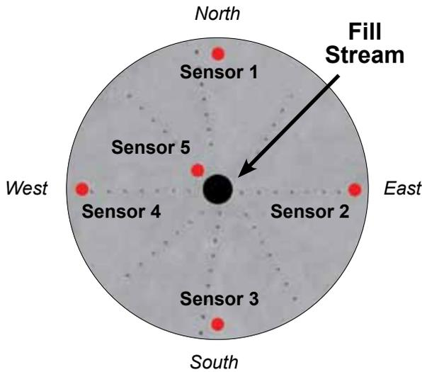
By installing multiple SmartBob sensors in the bin, it is also possible to detect if material is accumulating in one or more measurement points in the bin. In this example, there are four sensors mounted around the outer perimeter of the bin, each one-sixth the distance from the outer perimeter – with one sensor each on the north, south, east and west in equal distances from one another. The fifth SmartBob sensor is mounted near the center of the bin, but away from the fill stream.
