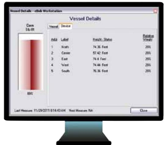
*These measurements indicate cone down and a higher level on the South sensor.*
