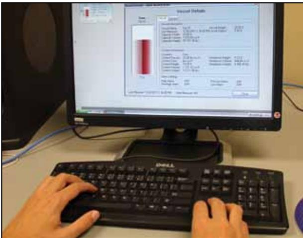
A percent value can be assigned to each sensor to prioritize the influence each sensor has on the average level. For example, the input from each sensor can be divided evenly so each sensor has an equal influence on the average level OR if the end user wants one or two sensors to have a greater influence on the average, a higher percentage of influence can be assigned. The total percentage for all sensors must always add up to 100 percent.
