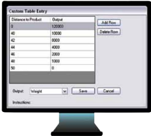
*Entering a custom strapping table is helpful in a non-linear vessel or in material that tends to compact.*
