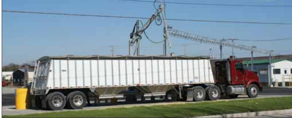
*New Intersystems truck probe takes a sample and sends it to the new scalehouse at right via pneumatic tube. Photo courtesy of Blanchard Valley Farmers Cooperative.*
