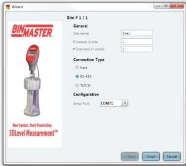
Figure 16: Project Wizard – Site Connection
