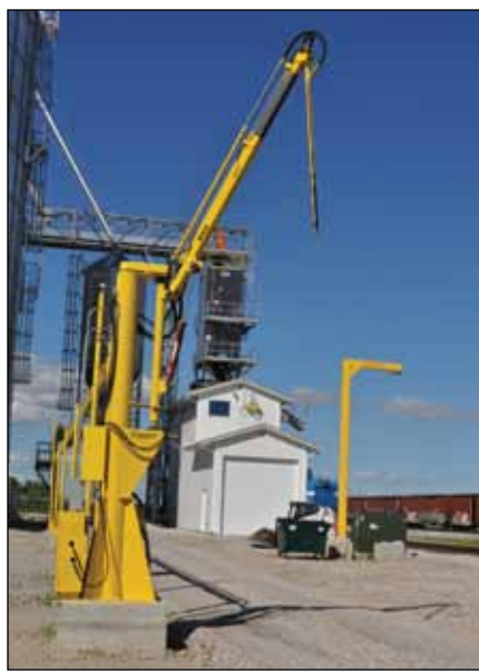
Grain handling equipment visible in this photo include a Gamet truck probe, Cardinal dump-through pit scale, and fall protection unit from CAI Safety Systems.
